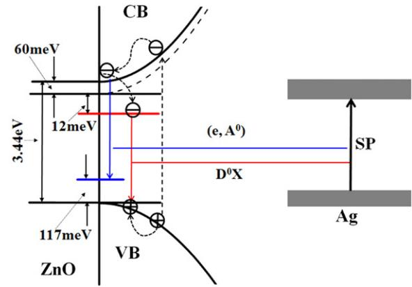
**Figure 3.** Schematic diagram of ZnO energy band structure and coupling processes of the SP in Ag with  $D^0X$  excitons and radiative dipoles in ZnO.
