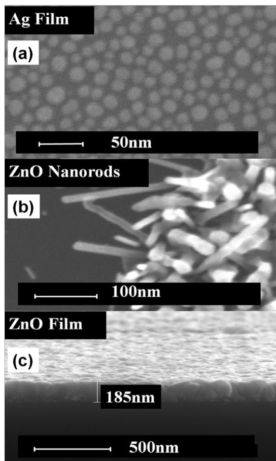
**Figure 1.** FE-SEM images of (a) the catalyst seed layer of 20 nm thin Ag film, (b) ZnO nanorods and (c) ZnO film.
